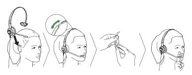
Jabra Biz 2400 II headets have adjustable headbands for all day wearing comfort and bendable 360° spin boom arms, so they can be easily adjusted without breaking. It is recommended to position the microphone close to your mouth (approx. two fingers width).
